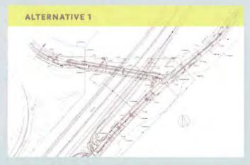
Alternative 1 provides a realigned Mulholland Bridge that intersects with Skirball Center Drive approximately 200 feet south of the existing intersection. The existing intersection of Mulholland Drive/Skirball Center Drive would be reconfigured to change eastbound and westbound through movements for Mulholland Drive into northbound and southbound through movements for Skirball Center Drive and Mulholland Drive.
