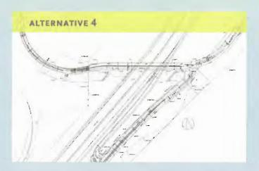
Alternative 4 provides a parallel, northerly aligned Mulholland Bridge that joins into existing Mulholland Drive approximately 150 feet north of the existing intersection, maintaining eastbound and westbound through movements for Mulholland Drive.
