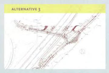
Alternative 3 provides a realigned Mulholland Bridge with a roundabout intersection of Mulholland Drive and Skirball Center Drive. The center of the roundabout wouldbe approximately 220 feet southwest of the existing intersection.
